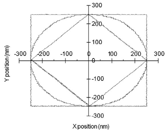
**Figure 5.** Example of trajectories made with our nanodisplacement system. The starting point is located at  $X = 0$  and  $Y = 250$  nm. Firstly, the system operates a circular path of 250 nm radius, then a square motion of the same size, and finally a diamond.
