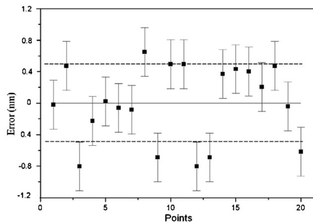
**Figure 6.** Repeatability for long-range displacements. A sequence of 20 back and forth displacements of 5 mm is launched. The straight line represents the mean value and the dotted lines the standard deviation which is equal to 0.5 nm.
