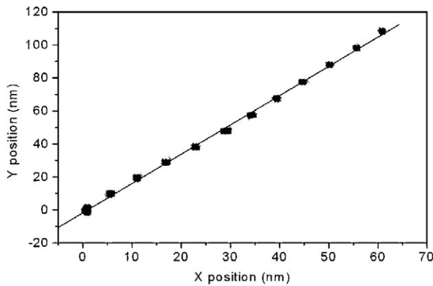
**Figure 4.** Displacement in an XY plane with 10 nm steps in the Y direction and 5.6 nm steps in the X direction. The low periodic discrepancy is due to the optical nonlinearities of the heterodyne interferometer.
