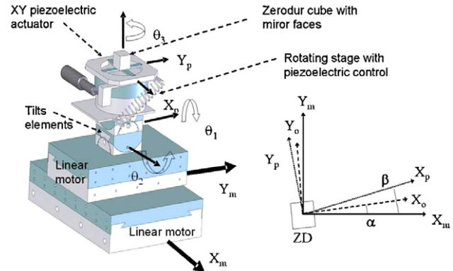
**Figure 3.** 3D overview of the system.  $(X_m; Y_m)$  are the displacement axes of the long-range stages;  $(X_p; Y_p)$  are the axes of the piezoelectric actuators;  $(X_o; Y_o)$  are the axes of the mirror cube. The angles  $\alpha$  and  $\beta$  are respectively the misalignment angles between  $(X_m; Y_m)$  and  $(X_o; Y_o)$  and between  $(X_m; Y_m)$  and  $(X_p; Y_p)$ .
