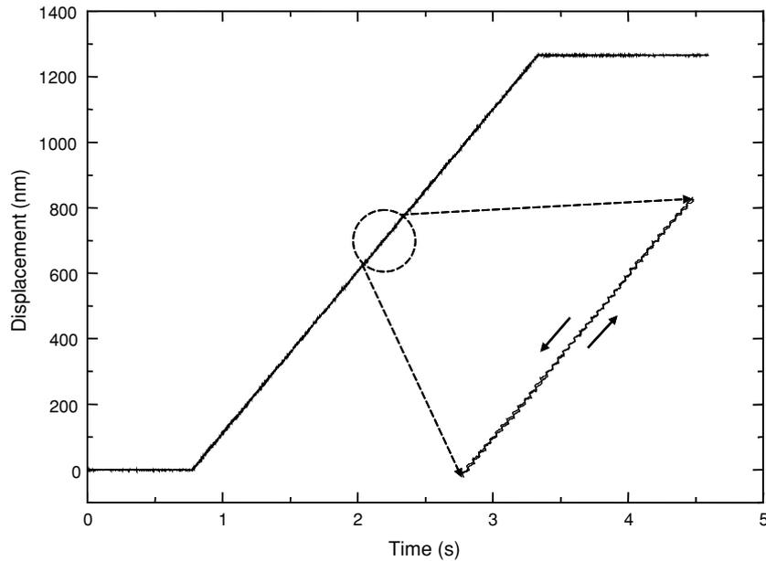
**Figure 8.** Hysteresis of the piezoelectric actuator used in the close mode. The centre of the curve has been zoomed over 200 nm.
