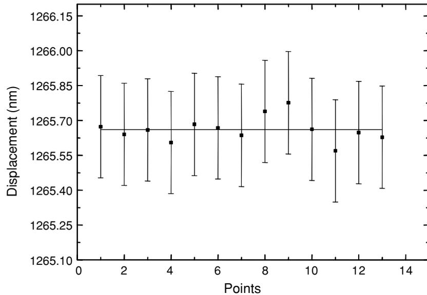
**Figure 6.** Repeatability of the method.  $K$  phase-shifts are programmed to generate a displacement of the target mirror from zero to  $x_B$ . The repeatability is given by the standard deviation of the set of the values of  $x_B$ . Straight line represents the mean value.
