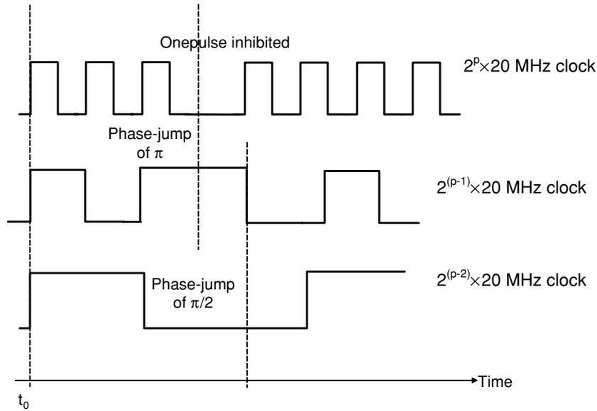
**Figure 2.** Principle for the generation of the phase-shifts. A high frequency clock generates a signal at a frequency of  $2^p \times 20$  MHz. Others signals are generated from this signal with a frequency divided by  $2^m$  with  $0 \leq m \leq p$ . An inhibition of one pulse of the primary clock corresponds to a phase-shift of  $2\pi/2m$  of the signal at a frequency of  $2^{p-m} \times 20$  MHz.
