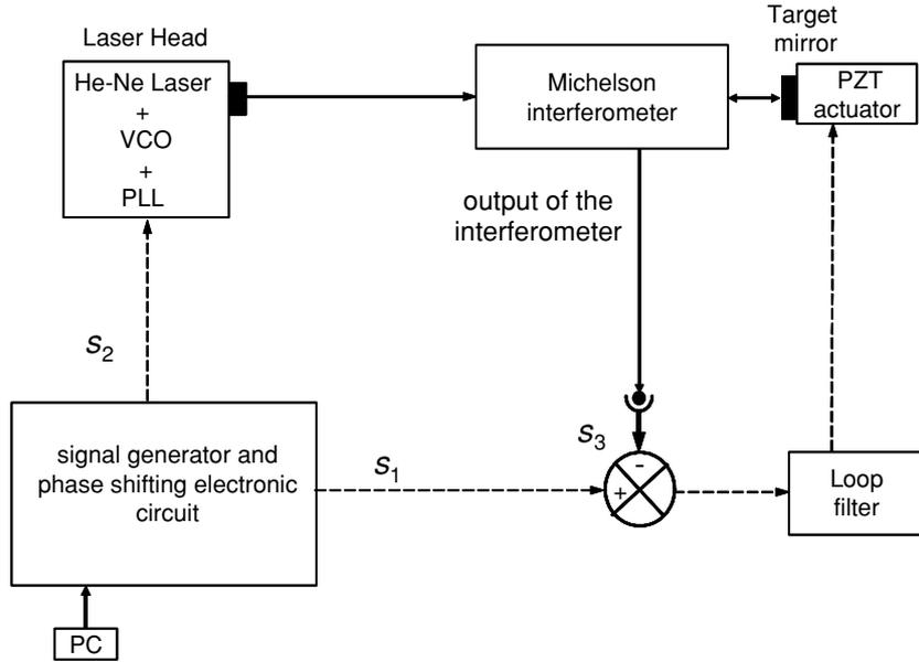
**Figure 1.** Principle of the position control method. A home-made electronic circuit puts out two synchronous signals both at a frequency of 20 MHz. A voltage controlled oscillator (VCO) in the laser head generates the heterodyne components of the laser source. This VCO is synchronized to the signal  $s_2$  thanks to a PLL system. The other signal ( $s_1$ ) is sent to a mixer to be phase compared with the signal  $s_3$  coming from the output of the interferometer.
