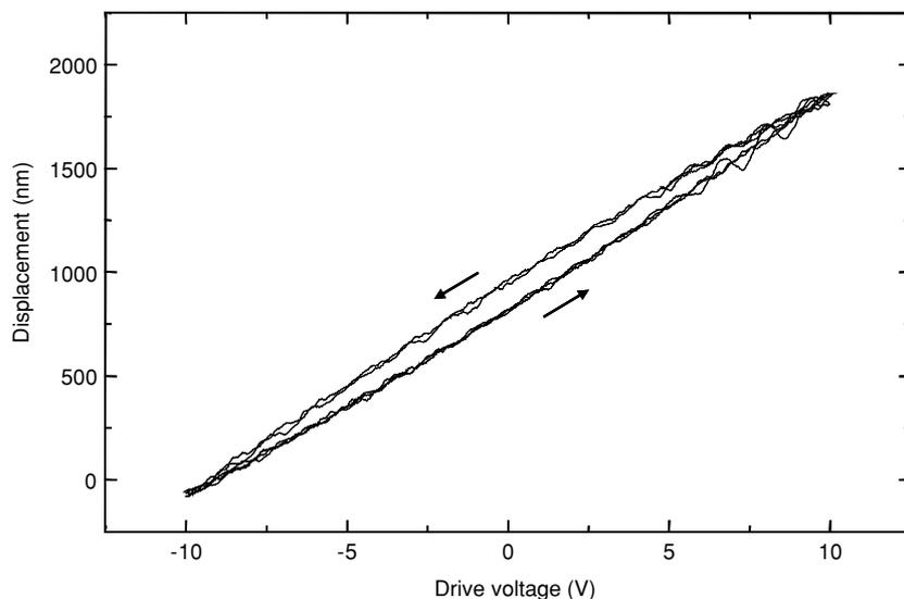
**Figure 7.** Hysteresis of the piezoelectric actuator used in our experiment in the open mode.
