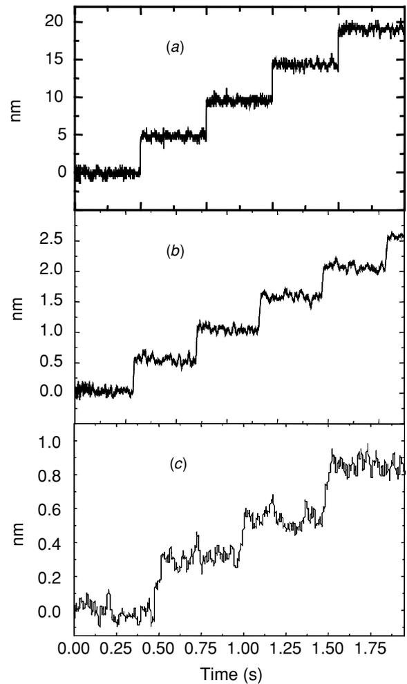
Figure 5. Experimental results. According to the values of  $p$  and  $q$ , different steps of the piezoelectric actuator are realized. (a)  $p = 32$ ,  $q = 0$ ,  $\Delta x_1 = 4.945$  nm. (b)  $p = 32$ ,  $q = 36$ ,  $\Delta x_2 = 0.549$  nm. (c)  $p = 34$ ,  $q = 36$ ,  $\Delta x_3 = 0.259$  nm.
