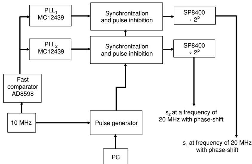
**Figure 3.** Sketch of the electronic board. Two synchronous high frequency clock, obtained from two phase locked loop MC12439, are synchronized to a 10 MHz reference quartz oscillator. Some positive emitter coupled logic components with working frequencies upper than 2 GHz and with very low phase noise characteristics are used to perform inhibitions and frequency divisions.
