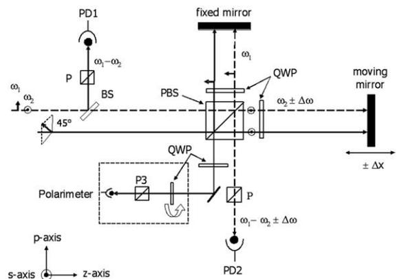
Fig. 1. Schematic representation of the principle of heterodyne (dash line) and homodyne (straight line) laser interferometers: P, polarizer; PBS, polarizing beamsplitter; PD, photodetector; BS, beamsplitter; QWP, quarter-waveplate.
