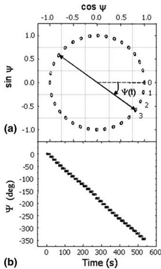
Fig. 7. Variation of  $\psi$  as a function of time (b) and in a Fresnel representation (a). Each group of points represents a displacement of the target mirror of  $\lambda/32 = 19.781$  nm.
