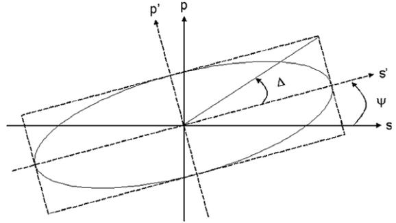
Fig. 2. Definition of the ellipsometric parameters  $\psi$  and  $\Delta$ .
