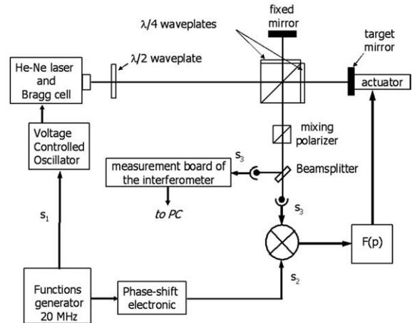
Fig. 3. Principle of the position-control method of the target mirror using a heterodyne laser interferometer.
