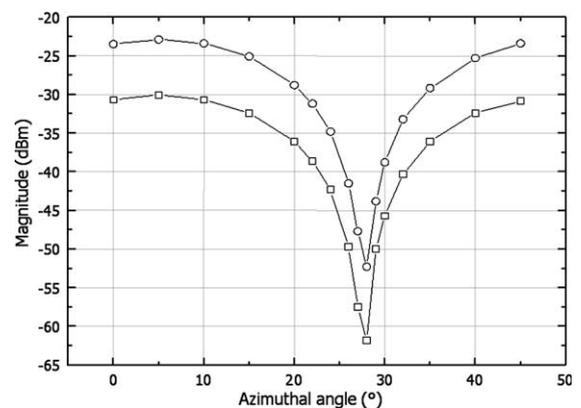
Fig. 6. Frequency spectrum of the signal at the output of the interferometer showing the magnitude of the residual optical beat frequency signal in each arm of the Michelson interferometer as a function of the azimuthal angle of the half-waveplate. Fixed arm (—O—); moving arm (—□—).
