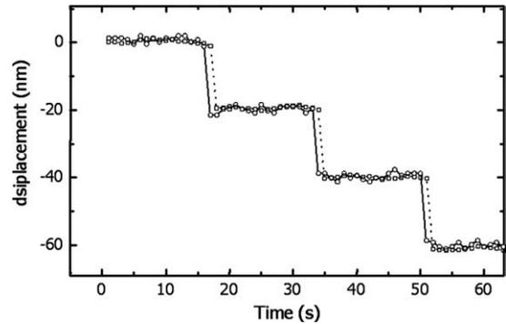
Fig. 4. Optical path changes measured with both interferometers (—○—) homodyne interferometer (—□—) heterodyne interferometer. The target mirror is displaced step by step with a known step of about 20 nm by a piezoelectric actuator.
