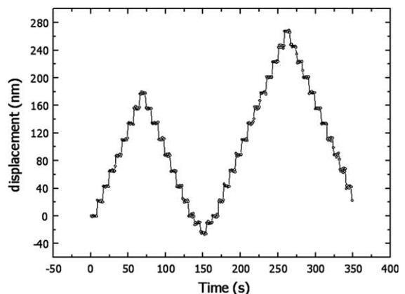
Fig. 5. Nanometric scale representation of the Kefren and Kheops pyramids using our polarimetric interferometer.
